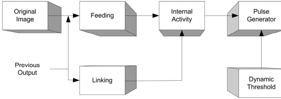
Fig. 1. Basic model of the PCNN.
